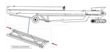
6. FOLD OUT CONVEYOR HEAD SECTION. UNIT IS NOW IN A WORKING POSITION.
